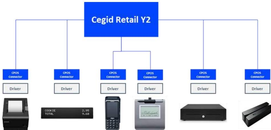
Instead of exchanging directly with each device, the POS terminal communicates with a generic multi-device connector called CPOS.
